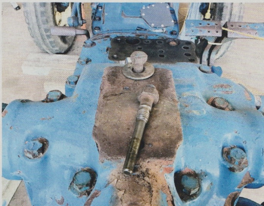
The peg stud that unscrewed out of the hydraulic top cover. It was beneficial that the three-point linkage had been removed and the peg stud could be threaded back in place after the nut had been removed.
